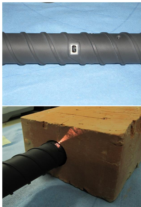
Slika 2: Ma-MISS – Mars Multispectral Imager for Subsurface Studies . Vir: Evropska vesoljska agencija, http://exploration.esa.int/mars/45103-rover-instruments/?fbodylongid=2133 .
